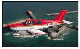
If the fixed-gear Tobago looks just like the retractable Trinidad, it should. The two share virtually identical fuselages, wings, tailfeathers and other major components.
